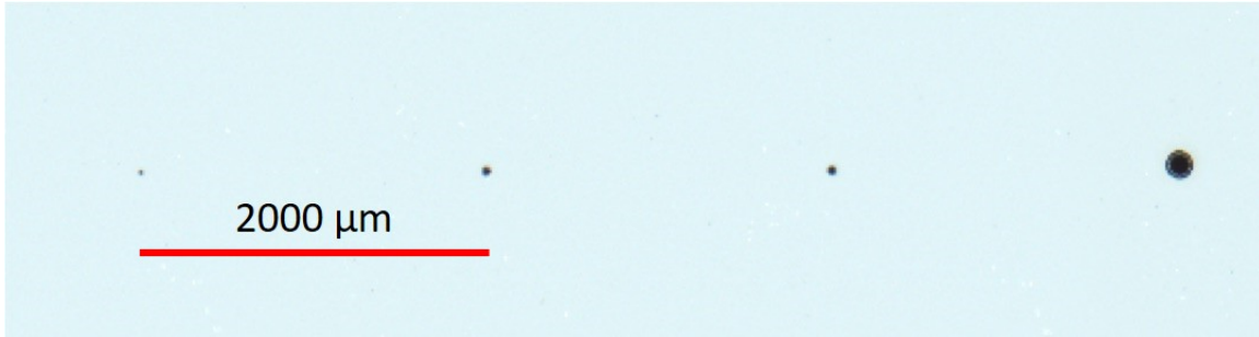
Figure 6. Craters from laser ablation in the heat conduction regime. \lambda = 1064 \text{ nm} , \tau_p = 10 \mu\text{s} , \omega_0 \approx 10 \mu\text{m} , F : varied, Material: Si, P = 1 \text{ atm} , T = 300 \text{ K} .
